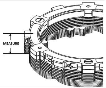
This measurement needs to be 1.343"-1.355" [34.1mm-34.4mm] tall. If it is taller than that, take out **1x** .048" [1.2mm] drive plate and replace with **1x** .040" [1mm] drive plate and remeasure. Repeat until the desired pack thickness is attained.
