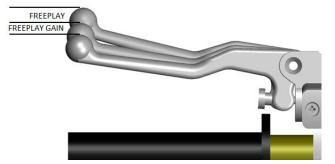
Optimal Free Play Gain yields **1/8" (3mm)** of clutch lever movement, measured at the end of the lever. This measurement at the lever correlates to achieving the ideal installed gap.
