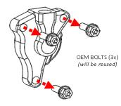
28. Mount the Rekluse slave cylinder to the engine using the OEM bolts.
