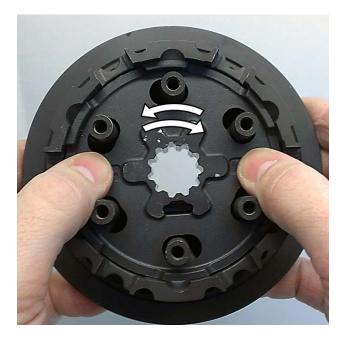
8. Remove the 6 rubber dampers from the OEM center hub assembly.
