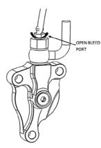
34. Slowly release the clutch lever and check the fluid level in the clutch master cylinder. Top off if necessary.
