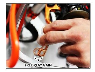
The following steps explain two ways to check Free Play Gain. One will use the rubber band that has been included in the clutch kit and one explains using your hand, which you will perform before every ride.
