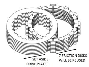
4. Inspect the friction disks for signs of heat or wear. Replace if they are burnt or worn with **KTM Part #: 59032011100**.
