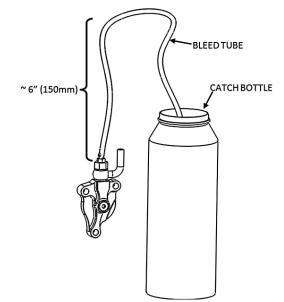
32. Pump the clutch lever 3-5 times then hold it against the bar/grip.
