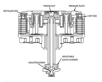
1. Using the long end of a 4mm Allen key, turn the adjuster screw clockwise until it stops under moderate pressure. You are trying to feel for the point at which the throw-out will start to lift the pressure plate. This is the "starting point."
