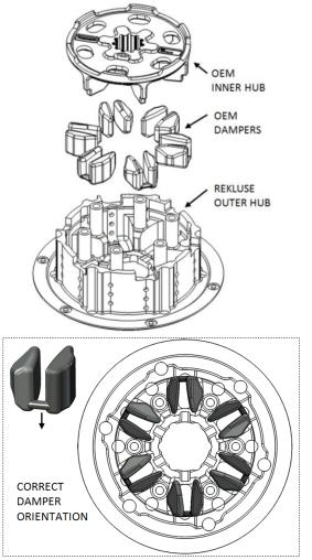
2. Install the new Center Hub Assembly into the clutch basket.
