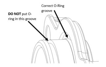
**NOTE:** The Rekluse slave cylinder comes preassembled in the kit. If the parts become separated, assemble them in the following order: Rekluse slave cylinder, O-ring, then the supplied paper gasket.
