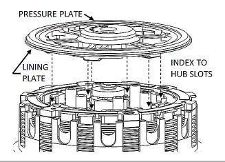
12. Install the OEM slider ring on the pressure plate with the "top" marking facing up. (The top side is rounded and the bottom edge is sharp.)
