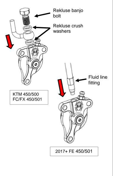
25. Tighten the banjo bolt (or fluid line fitting) with your hand until snug. (You will torque it to spec once installed on the bike.)
