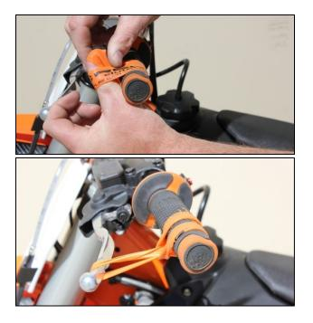
With the bike at idle in neutral, <u>quickly</u> blip (rev) the engine to at least 5,000 RPM and let it return to idle. The clutch lever should move in about 1/8" (3mm) toward the handlebar as you rev the engine. Turn the Slave Cylinder adjuster screw clockwise 1 tick at a time until optimal clutch lever movement (i.e. Free Play Gain) is achieved.
