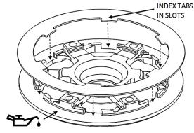
11. Install the pressure plate subassembly.
