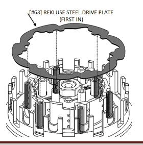
**NOTE:** Proper orientation of the drive plates is *critical* for optimal clutch performance. If you install them backwards, the clutch will still function but will lack proper modulation performance.
