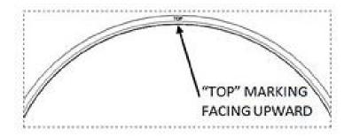
13. Place the OE Belleville spring onto the slider ring, with the rounded dome side facing up.
