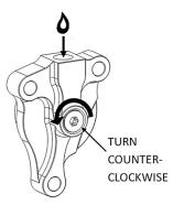
f. Compress the piston until it bottoms out. Repeat steps c – f until there is no longer air escaping from the top port when the piston is compressed.
