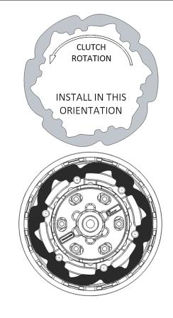
Install the rest of the clutch pack, using 8x Rekluse steel drive plates and 7x OEM friction disks in total.
