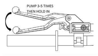
33. Using an 8mm wrench, open the bleed port. Air and fluid should come out of the bleed tube. Tighten the bleed port.
