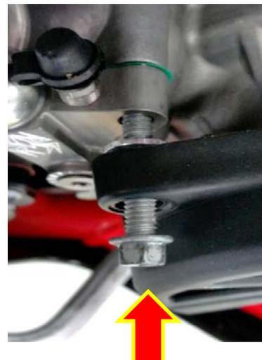
**NOTE:** The Rekluse screw sleeve is slightly taller than the OE screw sleeve. You will need to use the Rekluse screw sleeve to help ensure a good seal to the engine case.
