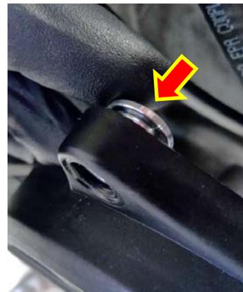
24. Reattach the chain guard to the slave cylinder using the longer OE screw.
