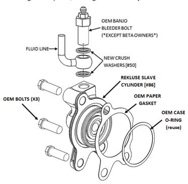
**NOTE:** Reuse the OEM paper gasket and OEM O-ring seal.
