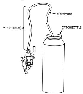
**23.** Pump the clutch lever 3-5 times then hold it against the bar/grip.
