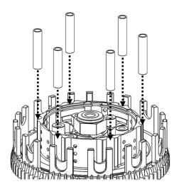
**8.** Install the first TEC drive plate in the orientation shown (all drive plates will follow this orientation).
