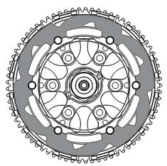
**9.** Install the rest of the clutch pack, noting the number and order of plates shown.
