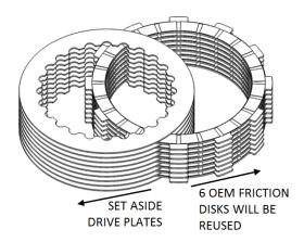
Inspect the friction disks for signs of heat or wear. Replace if they are burnt or worn.
