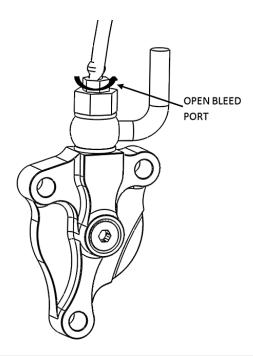
**25.** Slowly release the clutch lever and check the fluid level in the clutch master cylinder.
