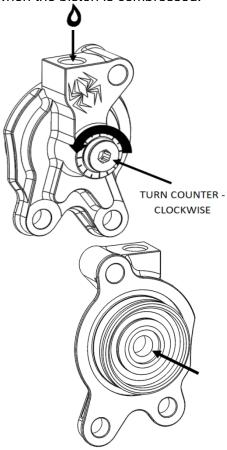
**NOTE:** When compressing the piston, fluid can shoot out from the slave cylinder port. Be sure to wear eye protection.
