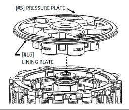
**13.** Install the Rekluse pressure plate springs and torque the pressure plate bolts.
