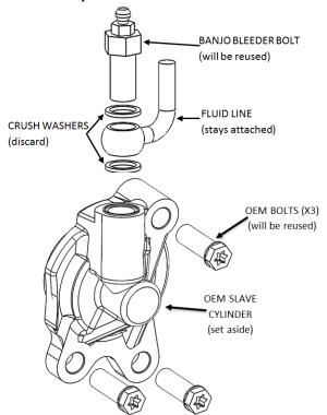
**17.** On a workbench (still away from the engine), bleed the Rekluse slave cylinder by this procedure:
