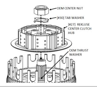
Torque the center clutch nut to 50 ft-lb (68 N-m), and bend up both tabs of the tab washer using channel-lock pliers.
