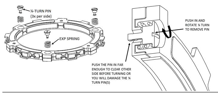
**CAUTION:** If you disassemble the EXP, bearing pads may fall out or be stuck to the ramp surfaces of the EXP bases. Take care to ensure all pads are correctly placed into wedge pockets using gentle pressure to avoid damage to the pad surfaces before reassembling the EXP. Properly seated pads will be secured in place once the EXP is reassembled. Operating the clutch without the pads in place will cause part damage or failure.
