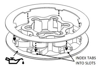
**12.** Install this pressure plate subassembly.
