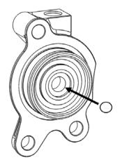
**19.** Install the Rekluse slave cylinder on the bike using these parts, ending with the banjo bolt.
