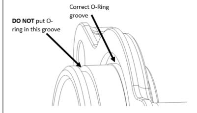
**NOTE:** Some models have a piston diaphragm seal. DO NOT REUSE them if OEM equipped.
