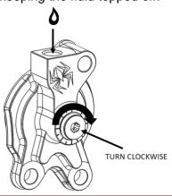
Turn the adjuster screw back to the initial position while compressing the piston until it bottoms out. Repeat this process until there is no longer air escaping from the top port when the piston is compressed.
