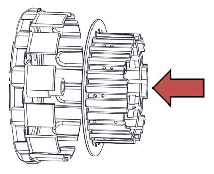
3. Install the new Rekluse tab washer with the bent tabs facing down, aligning with the holes in the hub. Only use the supplied lock tab washer under the OE center clutch nut when installing the hub.
