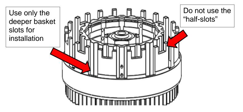
1. If a friction disk was included with your kit, place the included friction disk in engine oil to soak for at least 5 minutes.
