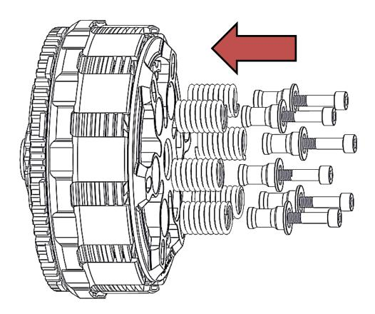
5.Use a torque wrench and socket to torque the cap screws by lightly tightening the screws in small increments. Torque the cap screws to 9 ft-lb (12 N-m).
