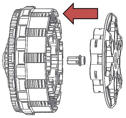
4. Install the pressure plate springs, followed by the screw sleeves and socket head cap screws (5 or 6 depending on the bike). Alternative spring options are available from Rekluse if desired. The springs provided are the recommended setting for optimum balance of performance and lever feel.
