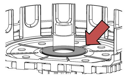
2. Install the new Rekluse center hub into the clutch basket.
