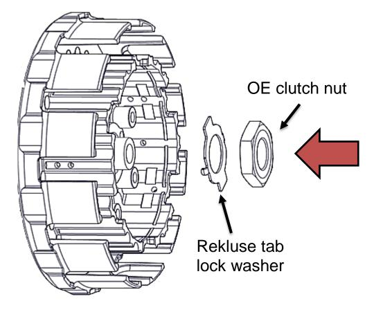
5. Using the socket and torque wrench, torque the center clutch nut to **50** ft-lb (**68** N-m).
