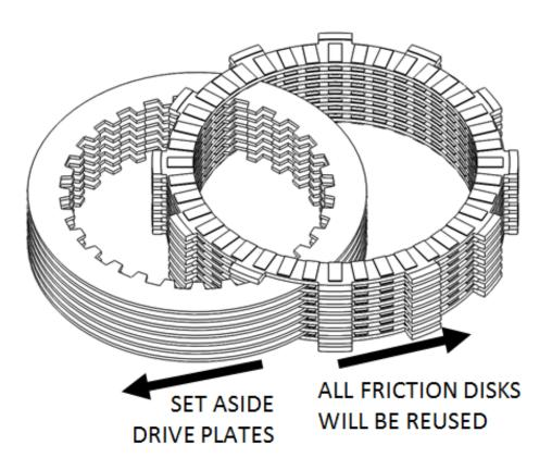
7. Inspect the friction disks for signs of heat or wear. Replace if they are burnt or worn.
