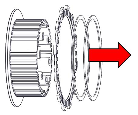
6.Separate the OE clutch pack. All the friction disks will be reused. All the drive plates will be replaced with Rekluse steel drive plates.
