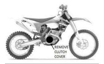
**3.** Remove the OEM clutch parts named in the following diagram down to the thrust washer. Leave the thrust washer installed in the basket.
