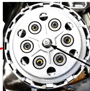
THROWOUT (LIFTS PRESSURE PLATE TO DISENGAGE CLUTCH)
