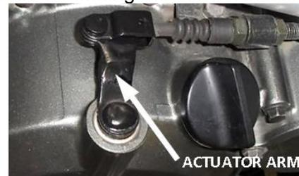
22. In the next section you will make adjustments using the front jam nut and perch adjuster to set the desired Installed-Gap based on the lever free play gain. Once this is established and everything functions well, you will tighten the rear jam nut to secure your cable adjustment setting.
