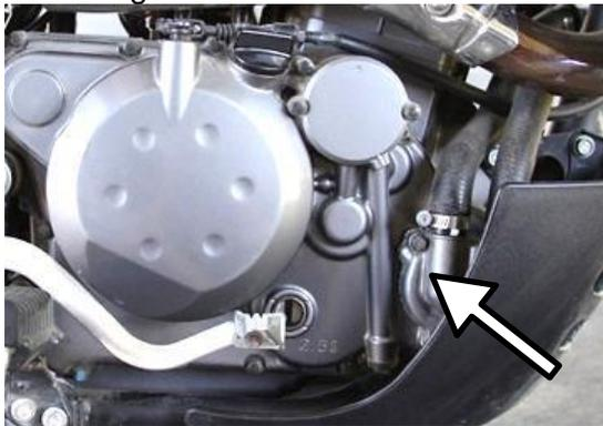
6. Using a 10mm socket, remove the water pump impeller nut. While removing the impeller be sure to remove both flat washers, one behind the impeller nut and one behind the impeller.
