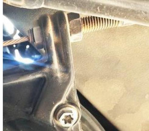
**Cause:** Possible stretched (worn out) cable, or possible incorrect clutch pack configuration.
