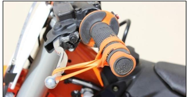
With the bike at idle in neutral, quickly blip (rev) the engine to at least half-throttle (~4,500 RPM) and let it return to idle. The end of the clutch lever should move in about 1/8" (3mm) toward the handlebar as you rev the engine.
