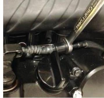
8. Using needle-nose pliers, grip and feed the clutch cable through the actuator arm to disconnect the clutch cable from the actuator.
