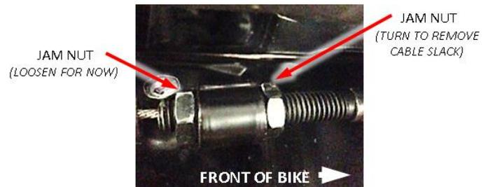
21. Once all the cable slack is gone, tighten the front jam nut about 3 more turns, so that the clutch actuator arm starts to move. This is a decent starting point for finding the correct installed gap.
