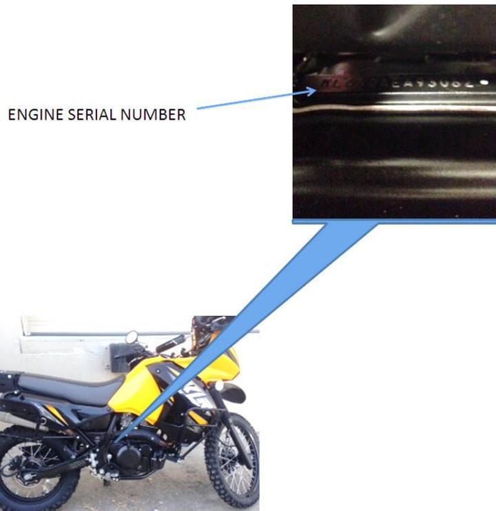
*Engine serial number is located just above the clutch cover and underneath the exhaust on the top surface of the engine.*
