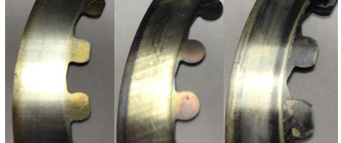
Normal Heat (Brownish) High Heat (Blue, Purple) Excessive Heat (Black)
